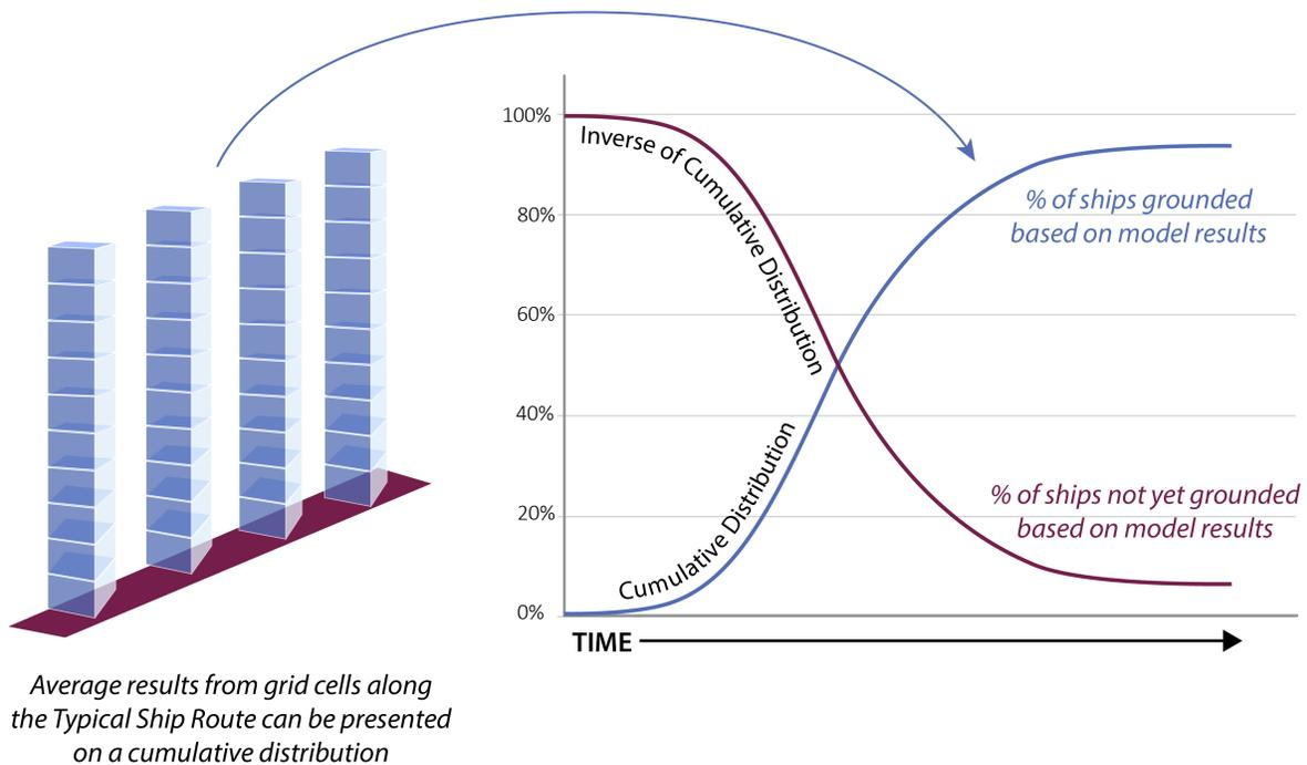
Figure 3-8: Cumulative distribution of the averaged results from model runs along the typical ship route in each focus area; shown also with the inverse of the curve which is used in the results
