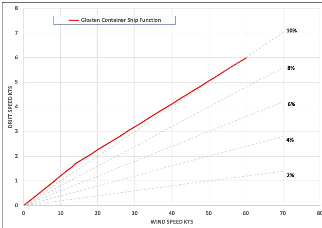
Figure 3-4: Plot of drift function (drift speed vs. wind speed) for a 7,500 TEU containership developed by The Glosten Associates (2013).
