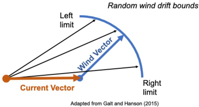
Figure 3-5: Graphical depiction of how the ZONS model incorporates current and wind data to estimate the direction and speed a ship may drift
