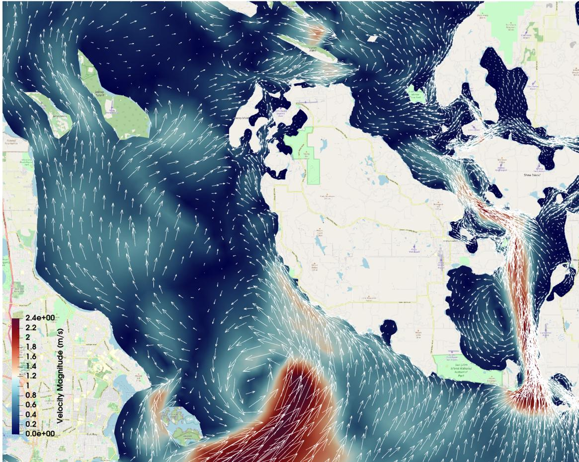
Figure 3-3: Predicted surface currents distribution from SSM on 1/1/2017 2:00:00 AM
