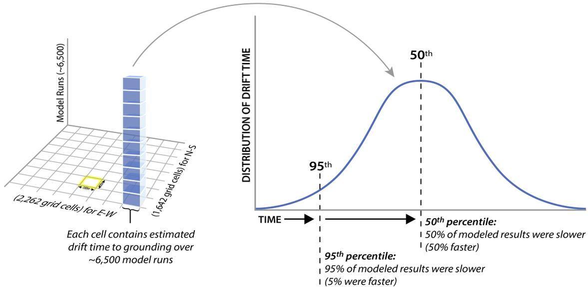
Figure 3-6: Simplified depiction of how the ZONS drift model results is generated
