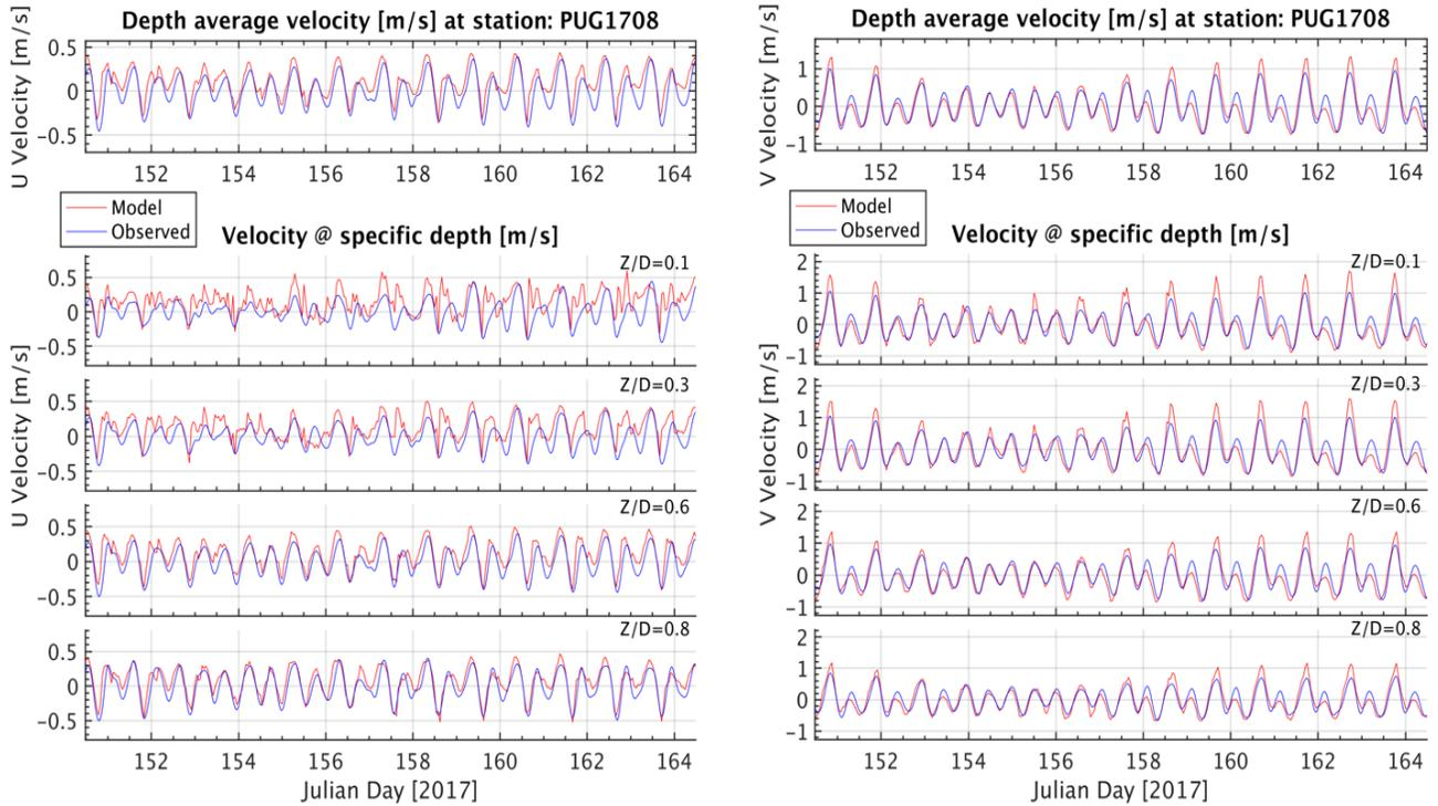
Figure 3-2: Comparison of predicted currents from the SSM to observed current data at a single station in 2017
